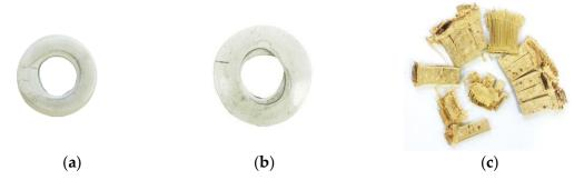
**Figure 6.** Shape of tube after deformation: (a) PVC Ø 20 (b) PVC Ø 25 and (c) Bamboo.
