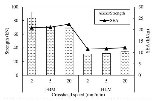
**Figure 14.** Compressive strength and SEA for FBM and HLM structure with three different compression crosshead speed.
