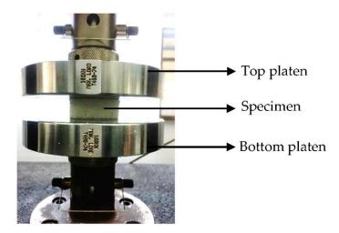
Figure 2. Quasi-static compression testing of specimen.
