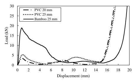
Figure 4. Load-displacement curves for three types of tube.
