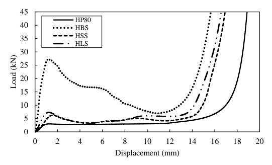
Figure 8. Load-displacement curve for HP80 reinforced with different type of single tubes.
