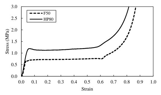
Figure 3. Stress-strain curves of F50 and HP80 foam.
