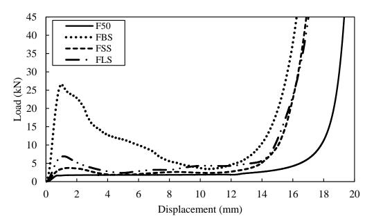
Figure 7. Load-displacement curve for F50 reinforced with different type of single tubes.
