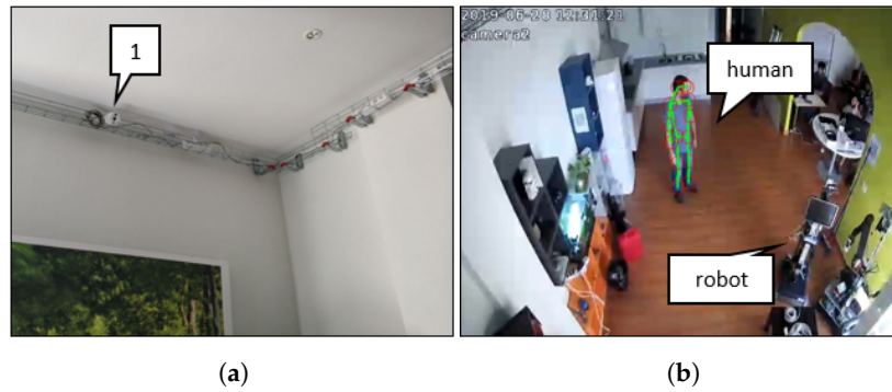
Figure 3. (a) Partial view of the physical world \mathbb{W} with an RGB camera with wired communication; and (b) image capture from the camera labeled as “1” in (a).
