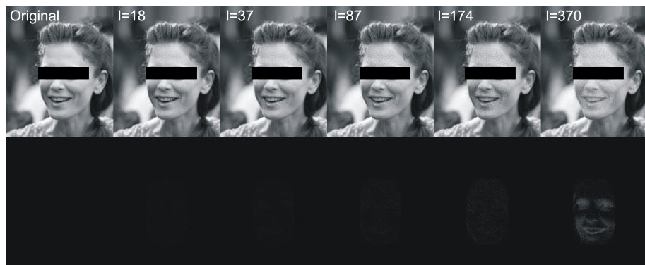
Figure 11. This figure shows an exemplary original image and images with hidden data of various lengths (first row) and differences between original image and images with hidden data of various lengths (bottom row). The threshold parameter for mixing (19) was set to t = 0.6 .
