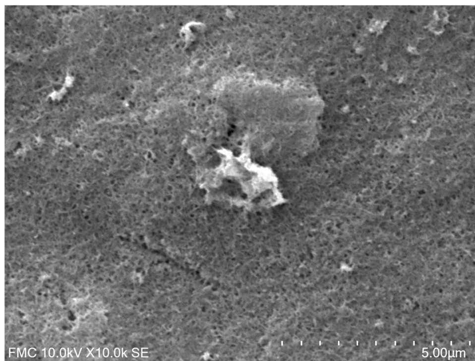
Figure 3. Scanning electron micrograph of the active surface of CNT-GNP-Lac/SPE.
