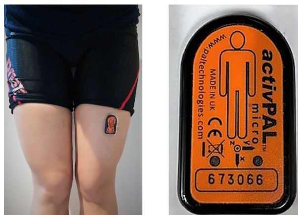
Fig. 3. Postoperative activity monitoring in total hip arthroplasty patients. Daily step counts were taken for one week using an accelerometer-based activity monitor (activPAL3). A front view of the thumb-sized monitor placed on the anterior aspect of the mid-thigh using a surgical dressing is shown.
