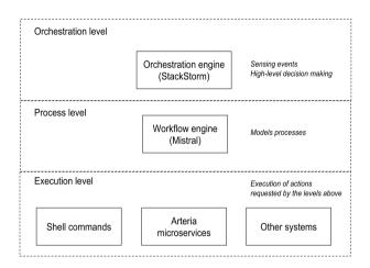
Figure 1: An overview of the conceptual levels of the Arteria project.
