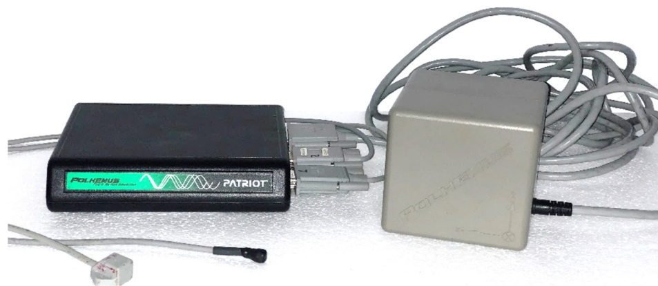
Figure 1. Polhemus Fastrak system. From left to right: receiver module, two sensors, emitter module.
