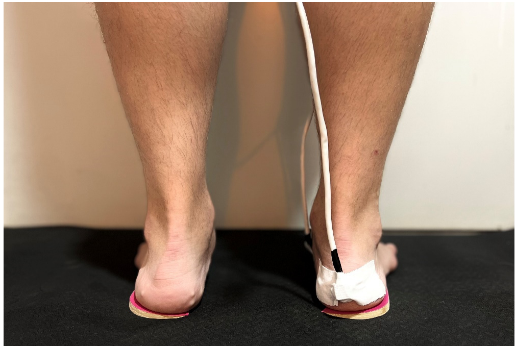
Figure 3. LWIs were placed under the calcaneus bones of both feet.
