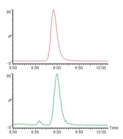
**Figure 1.** HPLC-MS/MS chromatograms of acrylamide-d3 (**top**) and acrylamide (**bottom**) in Black Japonica flatbread ( $50.5 \pm 6.1 \,\mu\text{g/kg}$ ). Y-axis: intensity; x-axis: retention time (min).
