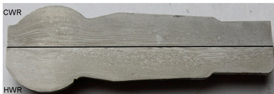
Figure 13. Material flow lines observed after etching in Jacewicz's reagent ( 38\text{ cm}^3\text{ HCL} + 12\text{ cm}^3\text{ H}_2\text{SO}_4 (1.83\text{ g/cm}^3) + 50\text{ cm}^3\text{ H}_2\text{O} ).
