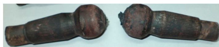
Figure 5. Ball studs after cutting during cross-wedge rolling (CWR).
