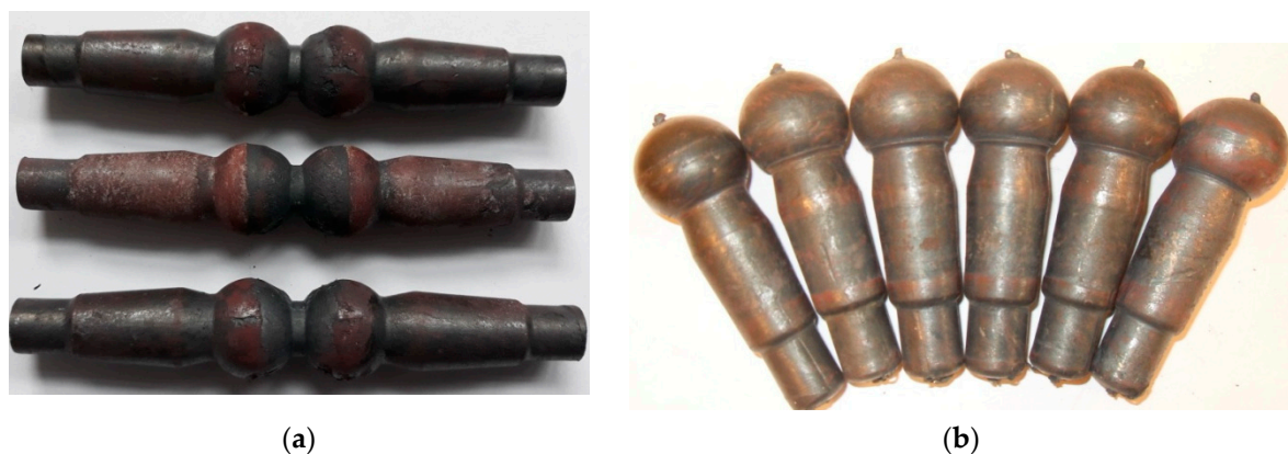
Figure 4. Ball studs obtained by: (a) cross-wedge rolling (CWR); (b) helical-wedge rolling (HWR).
