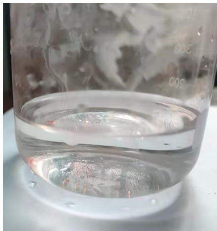
Figure 14. Result of oil-water separation.
