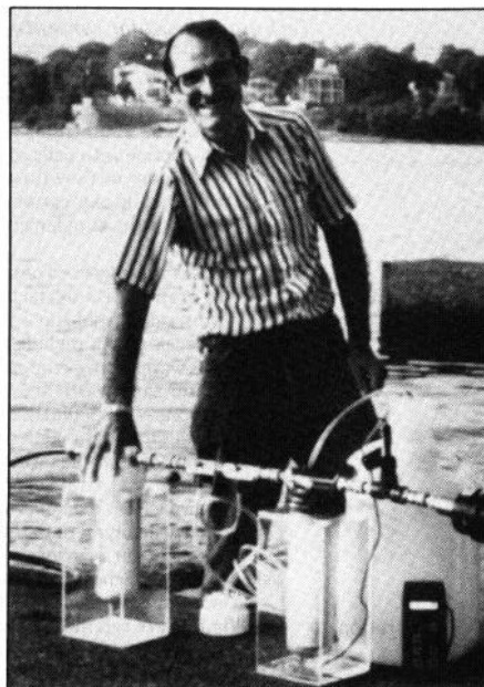
Viruses were concentrated from river water by directed adsorption onto a pleated membrane cartridge filter.
