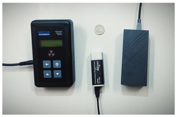
**Figure 2.** The radiological sensors used in this work. From left to right: the Mazur PRM-9000, the  $\mu$ SPEC 500 CZT, and the Sparkfun SEN-11345. A 1 euro coin is also present for scale.
