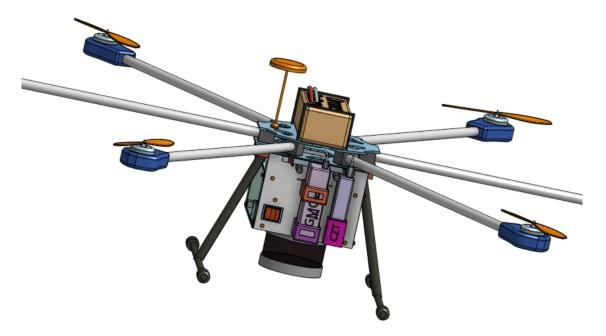
**Figure 12.** CAD image of the hexarotor and sensor-box underneath, encompassing GMC and CZT sensors as well as a LIDAR on the bottom.
