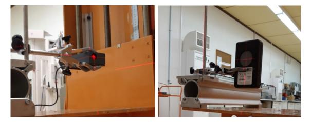
**Figure 4.** Acquisition setup for the Sparkfun (**left**) and the Mazur (**right**) verification procedure. The geometric center of the sensitive volume of each GMC was aligned with the source geometric center using vertical and horizontal lasers.
