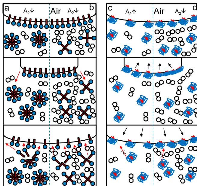
**Figure 5.** Schematic comparison of the impact of low (a,c) and high (b,d) sugar concentrations on the behavior of surfactants (a,b) and proteins (c,d) at the air–water interface.
