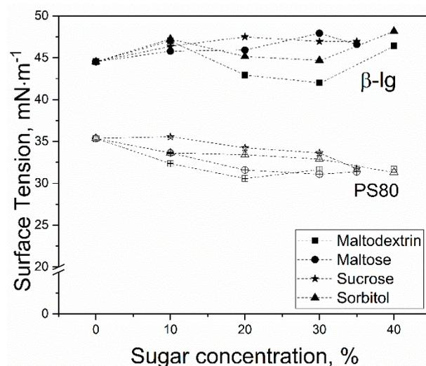
**Figure 1.** Surface tension of polysorbate 80 (empty symbols) and  $\beta$ -lactoglobulin (filled symbols) with different concentrations of added sugar after an equilibrium time of 7200 s at 20 °C, where (■) corresponds to maltodextrin, (●) to maltose, (★) to sucrose, and (▲) to sorbitol, respectively.
