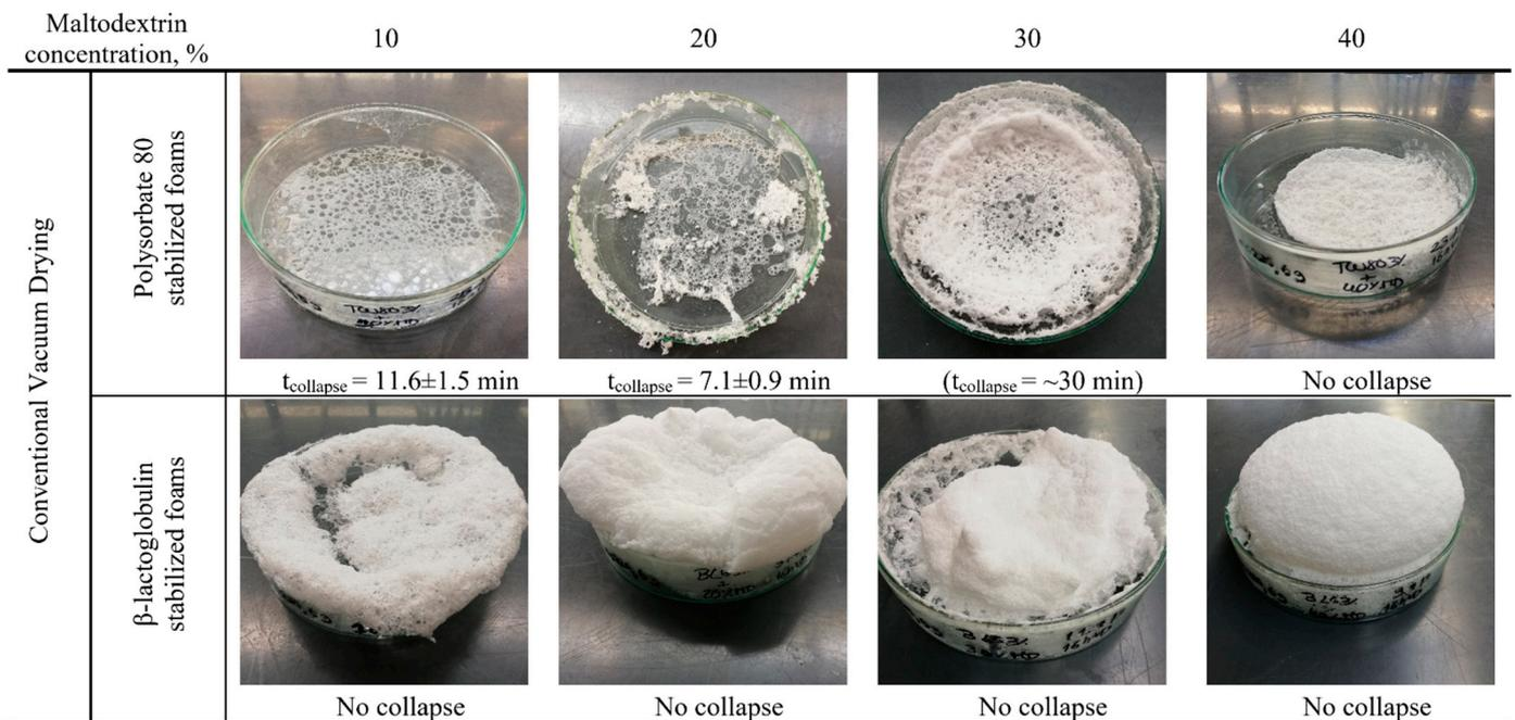
**Figure 7.** Foam structure after conventional vacuum drying for polysorbate 80 and  $\beta$ -lactoglobulin foam with a maltodextrin concentration between 10% and 40%.
