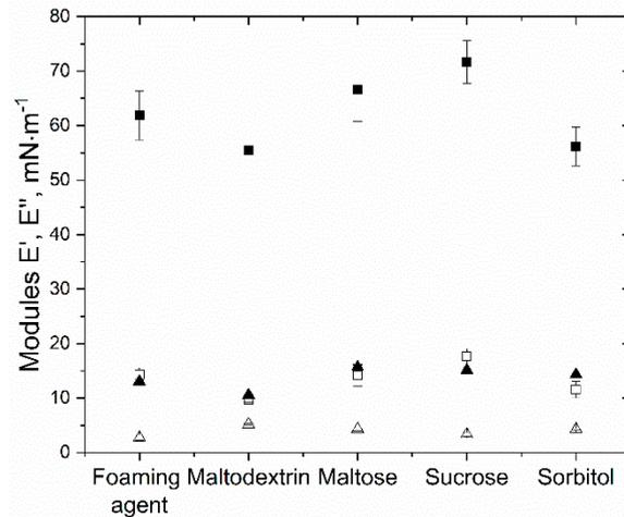
**Figure 2.** Influence of sugar type on the elastic ( $E'$ , squares) and viscoelastic ( $E''$ , triangles) moduli of polysorbate (empty symbols) and  $\beta$ -lactoglobulin (filled symbols) samples pure or with a saccharide concentration of 20%.
