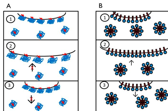
**Figure 3.** Schematic differences at the air–water interface between  $\beta$ -lactoglobulin (A) and polysorbate 80 (B) samples during oscillation.
