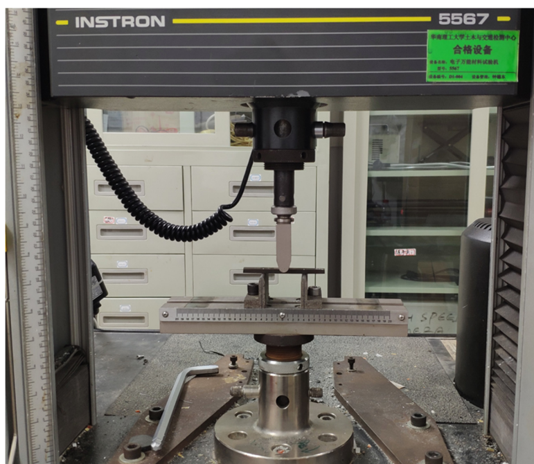
Figure 6. Three-point bending test of epoxy mortar specimens.
