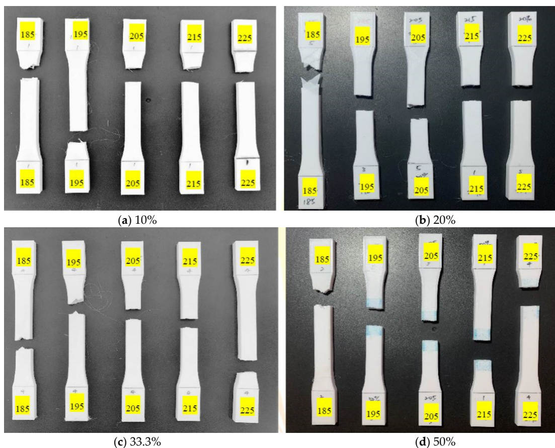
Figure 8. Tensile test specimens with different filling percentages (a) 10%, (b) 20%, (c) 33.3%, and (d) 50% under various printing temperature conditions after UV curing.
