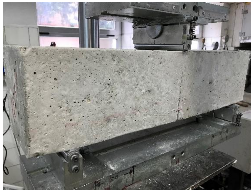
Figure 12. Location of the crack at the center span in one of the tested beams (Picture by authors).
