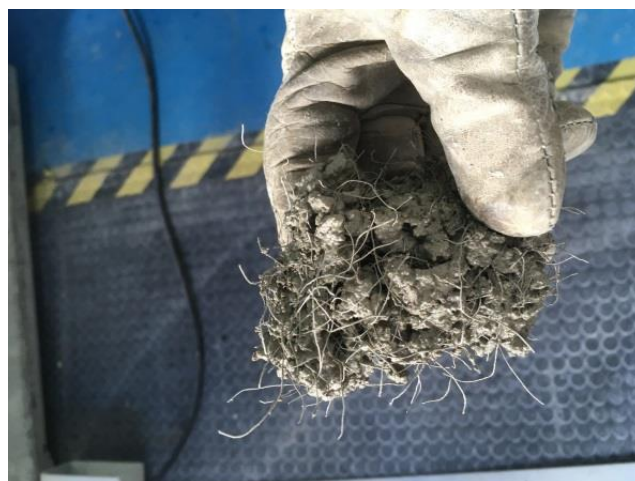
Figure 1. “Balling” effect of recycled steel fibers from tires (Picture by authors).
