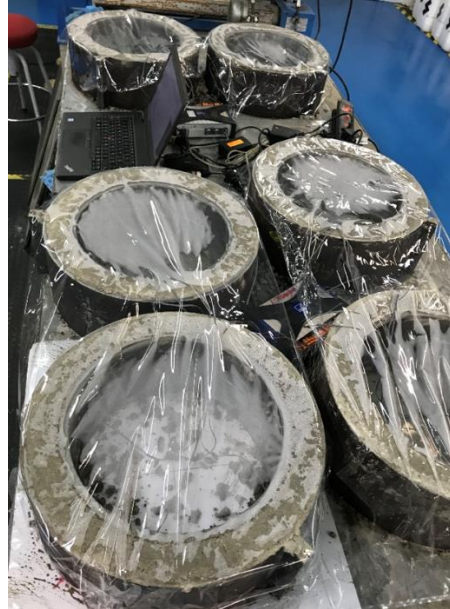
Figure 6. Concrete rings made to ascertain cracking resistance according to ASTM C1581 [57] (Picture by authors).
