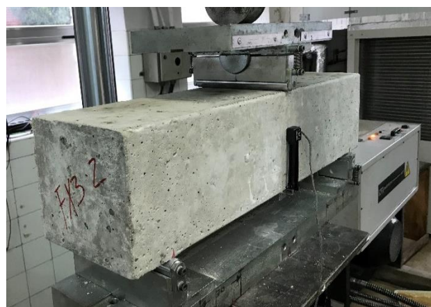
Figure 7. Test set up to ascertain flexural tensile strength according to EN 14651 [58] (Picture by authors).
