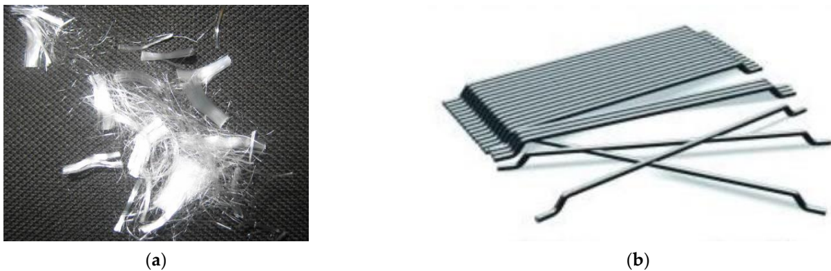
Figure 3. Common industrial fibers used in this paper: (a) polypropylene fibers; (b) steel fibers.
