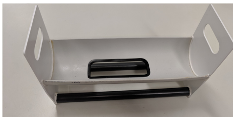
Fig. 1. Custom Cradle made from Poly Vinyl Chloride (PVC) 100 mm pipe with a 3 mm wall thickness.
