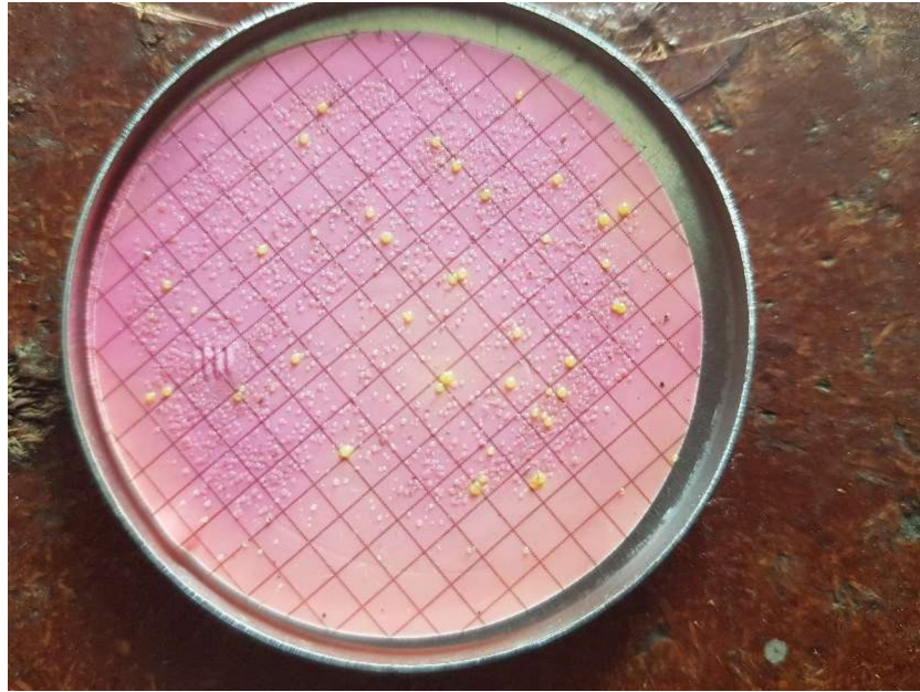
Fig 5. Growth of the thermotolerant microorganisms using membrane filter technique in water samples in Amhara and Afar regions of Ethiopia.
