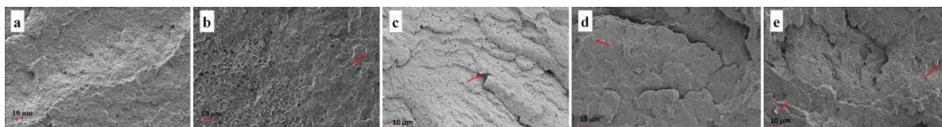
Figure 4. SEM images with magnification of 100 of nonfoamed samples of (a) as received neat co-PP; (b) 1 wt % xGnP incorporated nanocomposites via Method 1; (c) 2 wt % xGnP incorporated nanocomposites via Method 1; (d) 1 wt % xGnP incorporated nanocomposites via Method 2; (e) 2 wt % xGnP incorporated nanocomposites via Method 2. SEM: scanning electron microscopy, xGnP: graphene platelet.
