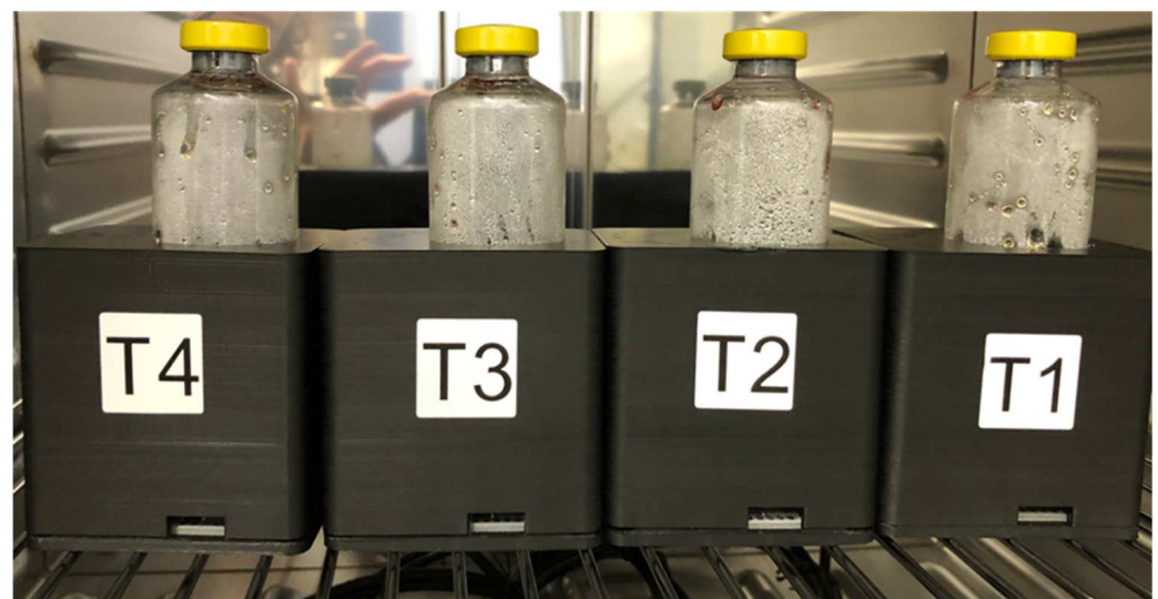
Figure 2. Setup of one growth experiment (1 run): three units of the turbidimeter prototype (T2-T3-T4) with BCBs containing spiked blood from the same “mother dilution” and one unit (T1) with a blank BCB (negative control, blood only). The BCBs in the turbidimeters are incubated in a dedicated incubator that remains closed during the growth experiment. Measurement data is then transferred to a laptop outside the incubator in real time, over a USB connection.
