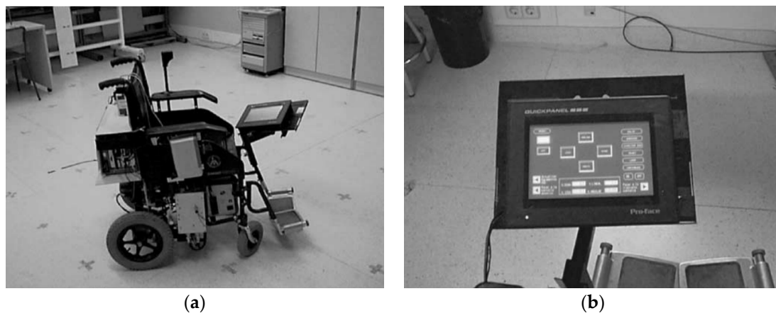
Figure 7. Wheelchair embedded with EOG input interface. (a) Overlook (b) Control display. Reprinted with permission from Ref. [15].
