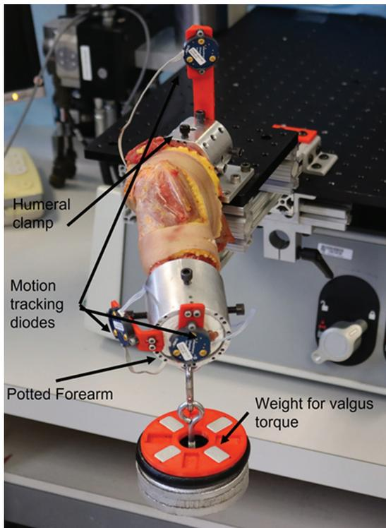
**Figure 3.** Kinematic testing setup. The humerus was clamped, and weights were added to the pot on the distal forearm to create a valgus load. Motion-tracking diodes were attached to the humerus and distal forearm. Each elbow was rotated from 10° to 120° of flexion, while valgus rotation of the forearm was recorded with respect to the fixed humerus.
