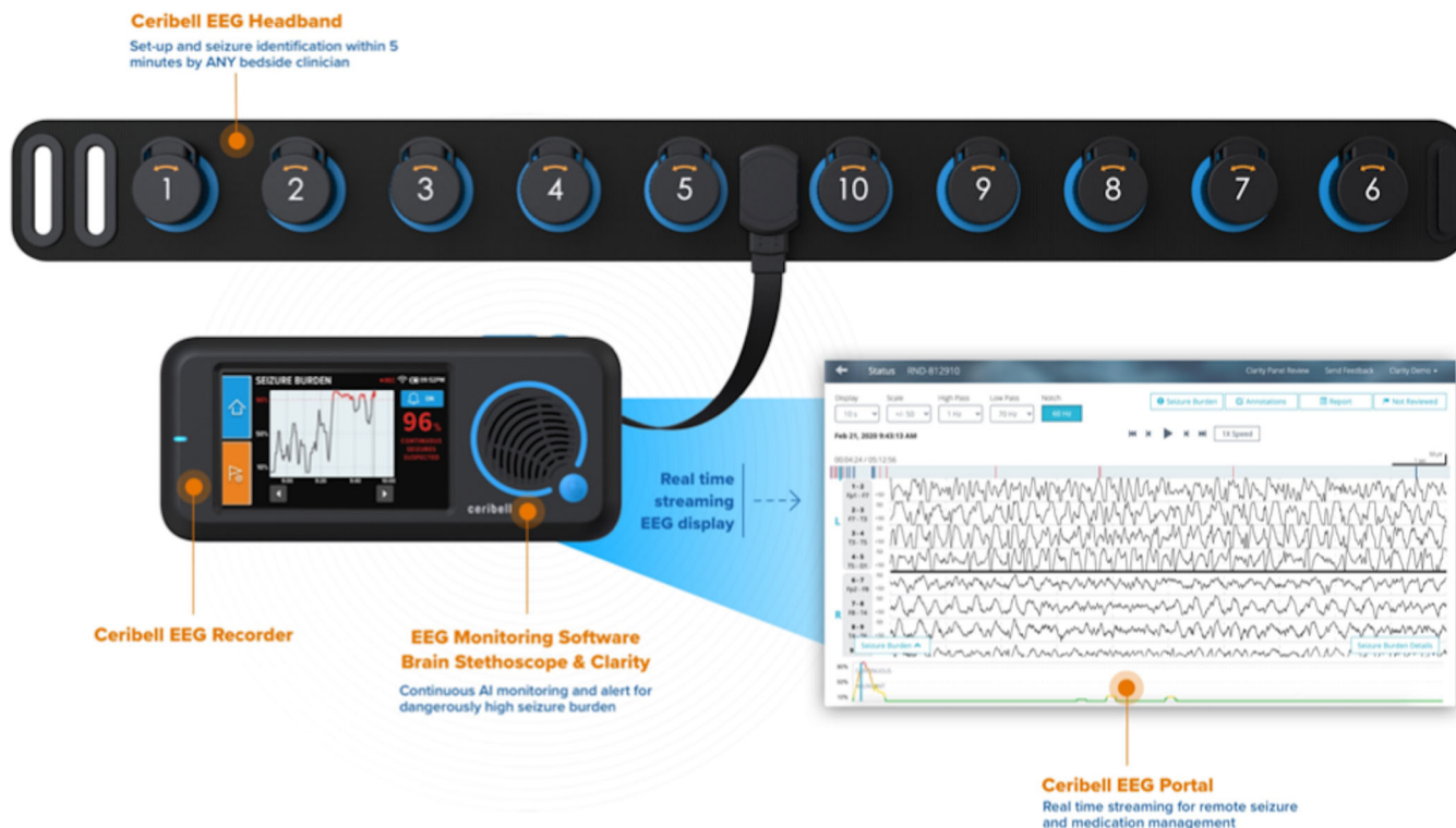
FIGURE 1 Ceribell point-of-care EEG. Rapid Response EEG is a point-of-care EEG system composed of a headband with 10 electrodes (corresponding to the temporal chains of the conventional 10–20 system) connected to a recorder that can be set up to record EEG data within minutes. EEG data can be reviewed at the bedside on the portable recorder using either the visual display of EEG waveforms or the audio output of the Brain Stethoscope function, which converts the waveforms from each hemisphere into an audible tone conveying rhythmicity and periodicity of brain activity in real-time. EEG data can also be reviewed remotely using an online portal. Rapid Response EEG is also equipped with Clarity, an artificial intelligence algorithm that continuously monitors the burden of seizure and seizure-like activity and displays a trend of seizure burden that is visible on both the bedside recorder and the online portal as well as an alert for impending status epilepticus when seizure burden reaches 4.5 minutes in any 5-minute period. Figure reproduced with permission from Ceribell Inc. ( www.ceribell.com ). Abbreviation: EEG, electroencephalography.
