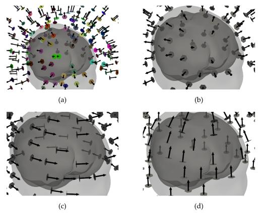
**Figure 2.** Different configurations of the SQUID measurement components for one selected subject: (a) the original Yokogawa system with 125 axial gradiometers magnetometers (SQUID-AXI-GRAD), (b) normal magnetometers (SQUID-NOR), (c) tangential magnetometers along the lines of latitude (SQUID-TAN-LAT) and (d) longitude (SQUID-TAN-LON). In the gradiometer system, the individual sensor pairs which form a gradiometer have the same color.
