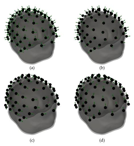
**Figure 1.** Different configurations of OPM-MEG for one selected subject: (**b**) normal components (OPM-NOR), (**c**) tangential components along lines of latitude (OPM-TAN-LAT), (**d**) longitude (OPM-TAN-LON) and (**a**) all three components combined (OPM-ALL). The gray surfaces show individual BEM mesh model layers. The center of the black dots represents the center of the OPM sensors, and the green arrows show the sensors' sensing directions. The sensor count for this subject is 93.
