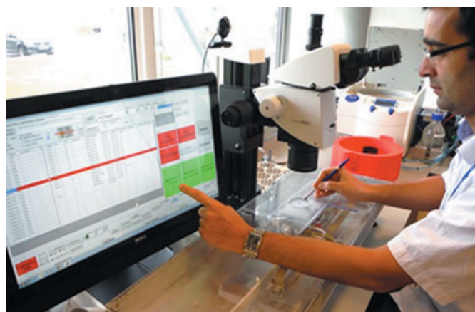
Figure 1 The Shifter at XChem. The operator is mounting through the mounting aperture, whilst operating the GUI with the free hand. The interface manoeuvres samples within the device enclosure, whilst automatically completing experimental annotations and documentation.
