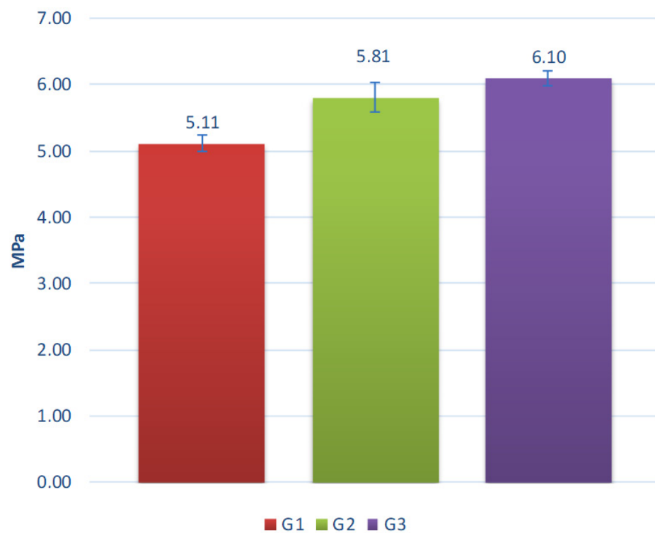
Figure 18. Crushing resistance of the aggregates after on 10% H 2 SO 4 water solution.
