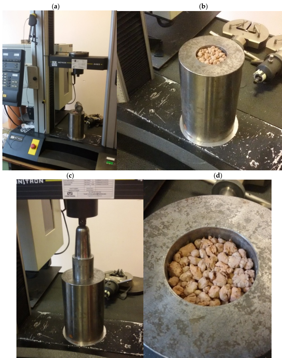
Figure 12. Testing stand for crushing of aggregates: (a) testing machine INSTRON 4469, (b) aggregate sample in steel cylinder before testing, (c) sample during loading, (d) sample after crushing test.
