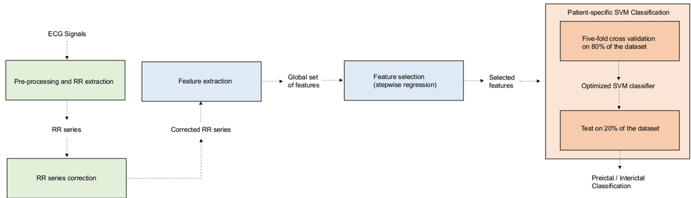
Fig 1. Flowchart of the proposed algorithm. The system consists of a pre-processing module, a feature extraction module, a feature selection module and finally a classification module based on Support Vector Machine. This last module includes a learning step, in which the classifier is trained, and a validation step, in which the optimized classifier is applied on the test set to classify preictal and ictal segments.
