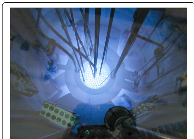
Figure 3 Triga nuclear reactor (1 MW) core with Cherenkov effect.
