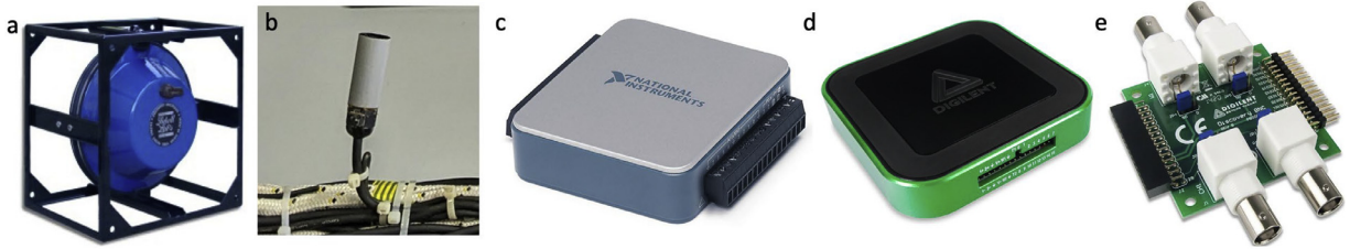
Fig. 4. Experimental setup for acoustic data acquisition. a) Underwater sound speaker Lubell LL-9162T, b) omnidirectional wideband hydrophone Benthowave BII-7017, c) analog-digital converter NI USB-6001, d) multi-instrument device Analog Discovery 3 with two analog input and two analog output channels connected via e) the BNC adaptor.
