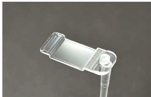
Figure 9. Injection compression molded MLA before the sprue is removed.
