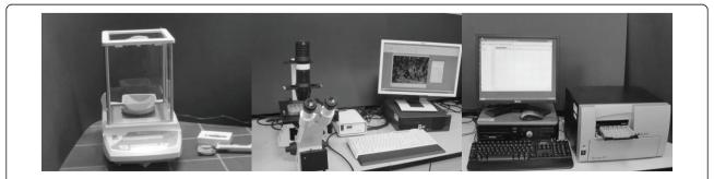
Figure 1 Analytical balance (Pioneer PA64, Ohaus, Pine Brook, USA), left; inverted fluorescence microscope (Axiovert 40C/Carl Zeiss, Göttingen, Germany), middle; fluorescence/luminescence reader (Synergy HT-Reader, Biotek, Winooski, VT, USA), right.
