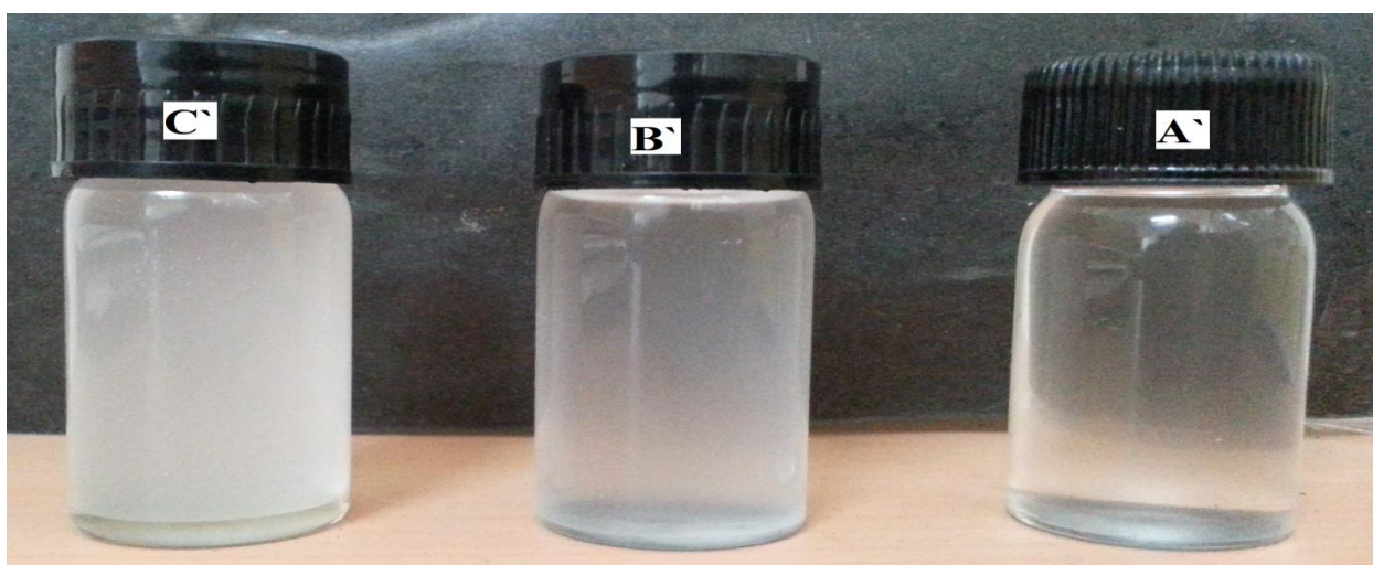
Figure 3. W/O microemulsion of Span 20, representing points (A') (clear microemulsion), (B') (slightly turbid microemulsion) and (C') (milky appearance microemulsion).
