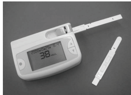
FIGURE 3: Portable sAA biosensor comprised hand-held reader and a disposable collector strip. Reprinted from [64] with permission from Elsevier.
