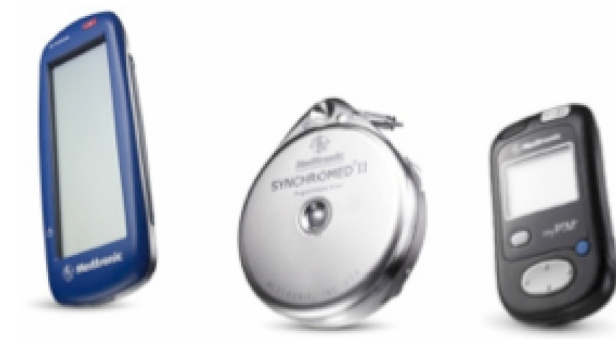
Figure 2 Medtronic SynchroMed II intrathecal pump, programmer, and patient therapy manager. Reprinted with the permission of Medtronic, Inc. © 2012.
