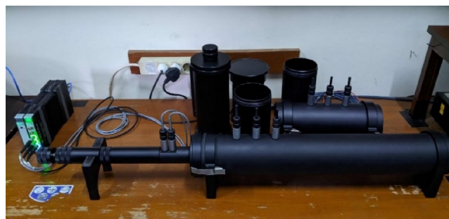
Figure 14. Measurement of SAC using the impedance tube.
