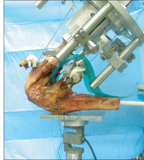
Fig. 6. Testing setup for quantifying the tibiofemoral contact and kinematics with kneeling.
