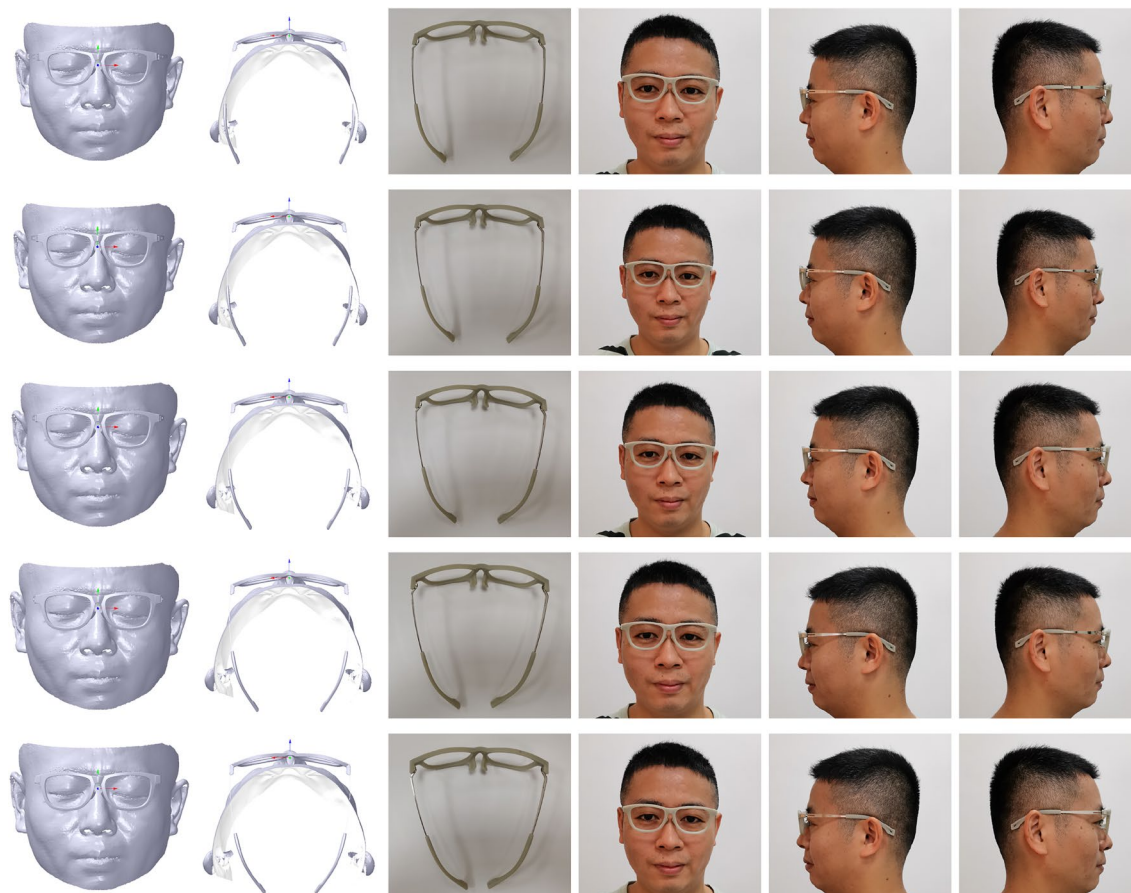
Figure 22. Try-on results of pile head rotation. From left to right: the front view, the vertical view, the printed glasses, the front view, the left view, the right view. From top to bottom: \beta with 3^\circ , 6^\circ , 9^\circ , 12^\circ and 15^\circ .
