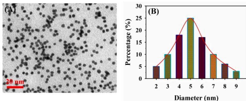
Fig. 2. TEM image (A) and size distribution (B) of Au nanoparticles.
