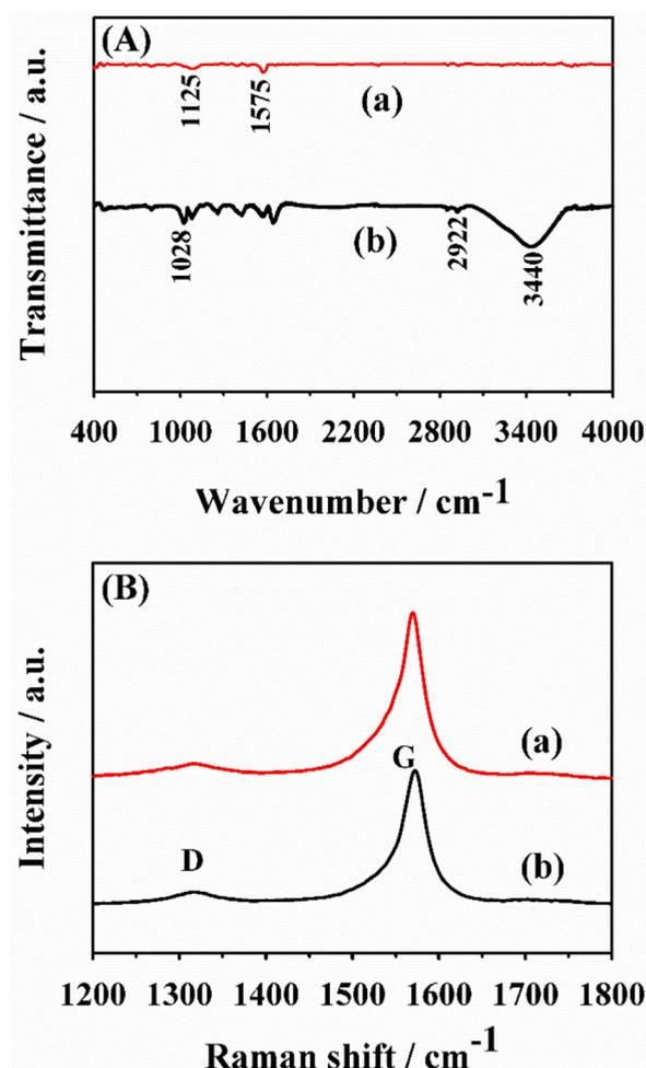
Fig. 3. (A) FT-IR and (B) Raman spectra of (a) CNTs and (b) CNTs-CD.
