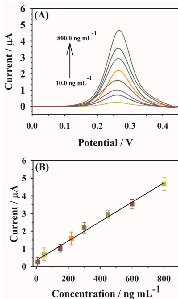
**Fig. 6.** (A) DPV responses of the design SEI assay at different concentrations of D-dimer (10.0–800.0  $\text{ng mL}^{-1}$ ); (B) the related calibration plot for D-dimer detection.
