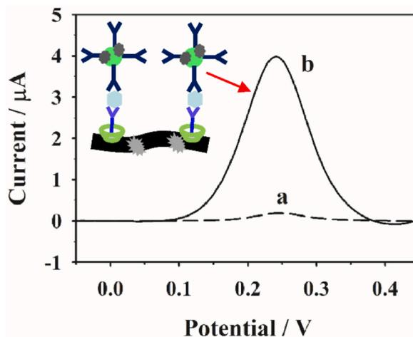
Fig. 4. DPV response of Ab<sub>1</sub>-CNTs-CD/GCE before (a) and after (b) its interaction with D-dimer and sequentially incubated in Ab<sub>2</sub>-Au-Fc solution.
