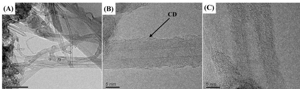
Fig. 1. TEM images of (A) CNTs and (B,C) CNTs-CD at different areas.
