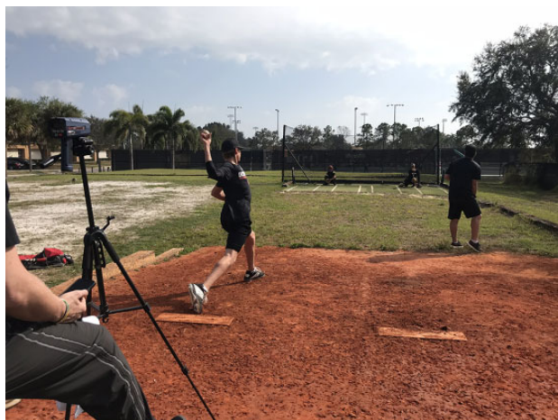
Figure 1. Pitchers throwing off the mound to a catcher at regulation distance (60.5 ft). The pitchers wore the sensor and sleeve, and ball velocity was tracked with a radar gun from behind the pitcher.
