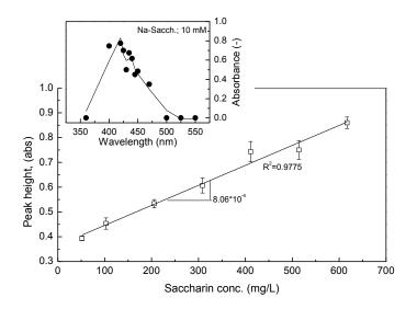
**Figure 2.** Linear calibration curve of saccharin under reference operating conditions (buffer flow rate and volume of 1.6 mL/min and 2400  $\mu$ L, respectively; 975  $\mu$ L of ethanol; 75  $\mu$ L of H<sub>2</sub>O<sub>2</sub> (7.10 M); 300  $\mu$ L of p-chloranil (20 mM); 150  $\mu$ L of saccharin).
