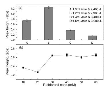
**Figure 3.** (**a**) Effects of the buffer flow rate and volume; and (**b**) effects of the p-chloranil concentration on the saccharin-SIA system under reference operating conditions with 10 mM sodium saccharin.
