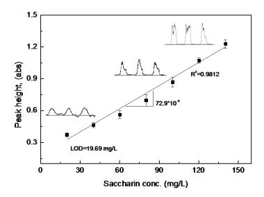
**Figure 5.** Calibration curve of a saccharin-SIA system under optimized operating conditions (buffer flow rate and volume of 1.2 mL/min and 2900  $\mu$ L, respectively; 870  $\mu$ L of ethanol; 30  $\mu$ L of H<sub>2</sub>O<sub>2</sub> (7.10 M); 150  $\mu$ L of p-chloranil (30 mM) and 450  $\mu$ L of saccharin).
