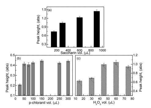
**Figure 4.** Effects of the reactant volumes on a saccharin-SIA system under reference operating conditions: (**a**) saccharin volume; (**b**) p-chloranil volume; and (**c**) hydrogen peroxide ( $H_2O_2$ ) volumes.
