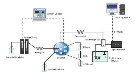
**Figure 1.** Schematic diagram of an sequential injection analysis (SIA) system for the determination of the saccharin concentration.
