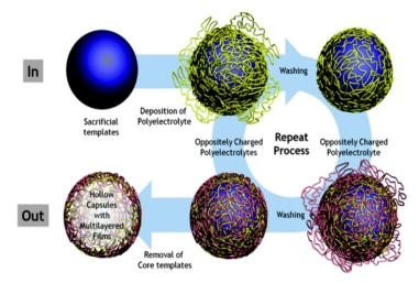
**Figure 2.** Schematic representation of polyelectrolyte multilayer capsules (PEMCs) formation using the polymer LbL deposition technique. This schematic is taken with permission from reference [119], copyright© 2011, Royal Society of Chemistry.
