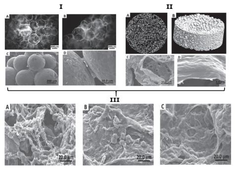
**Figure 14.** Images illustrating: (**I**) the interconnected PEMCs in 1D (A and B) and in 3D. (**II**) scaffold made of the PEMCs in 2D and 3D (A and B, respectively, from X-ray microtomography) and the internal structures of the scaffold (C and D). (**III**) SEM images of scaffolds with cells for cell culture after 24 h (A), 3 days (B), and 7 days (C). This figure is taken with permission from reference [221], copyright© 2010, John Wiley and Sons.
