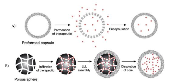
**Figure 6.** Schematics for the encapsulation of molecules of interest (e.g., bioactives) into hollow PEMCs: (A) loading into pre-formed PEMC and (B) incorporation into a porous sacrificial core utilized to assemble the PEMC. This figure is taken with permission from reference [163], copyright© 2006, Elsevier.
