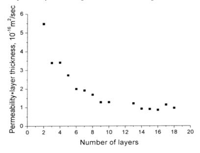
**Figure 9.** A graph showing the relationship between permeability and number of deposited layers, for (PSS/PAH) PEMCs, when fluorescein is encapsulated within. Permeability determined via the flux of fluorescein through the capsule wall. This figure is taken with permission from reference [203], copyright© 2001, American Chemical Society.
