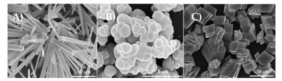
**Figure 4.** SEM images of three different polymorphs of CaCO<sub>3</sub> crystals: (**A**) aragonite; (**B**) vaterite and (**C**) calcite crystals. This figure is taken from reference [146], copyright© 2010, American Chemical Society.
