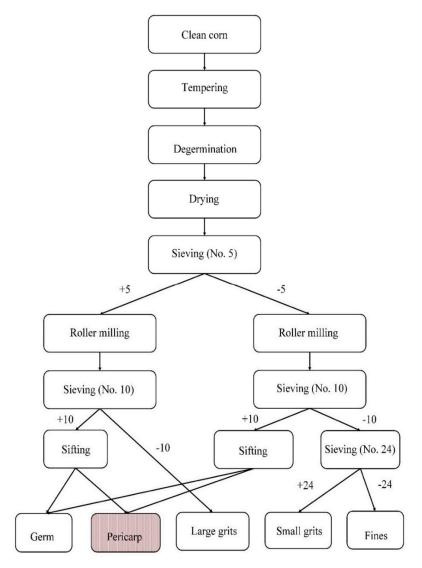
**Figure 1.** Process schematic of lab-scale dry milling protocol. The numerals represent the size of screen used, and + and – symbols represent the fractions recovered at the top and under those sieves, respectively (adapted from Rausch 2009) [64].
