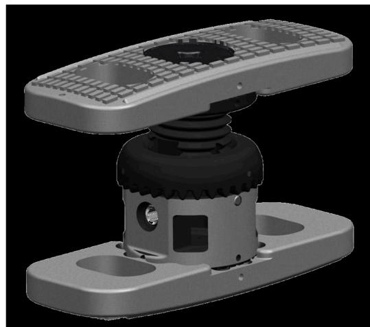
Figure 3. Prototype of the non-metallic, X-ray-translucent CF/PEEK expandable VBR. icotec, Altstätten, Switzerland.
