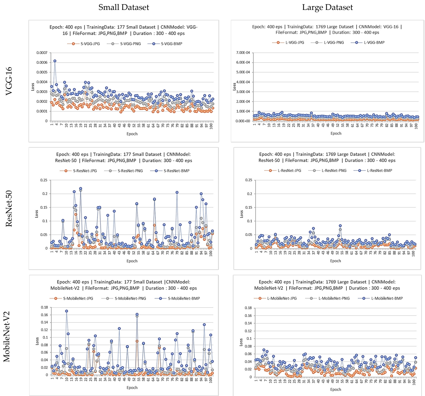
Figure 7. Training graph between 300 to 400 epochs of 18 CNN models trained by the small (left) and large (right) dataset.
