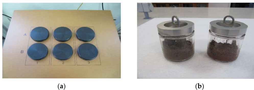
Figure 1. (a) Profiles of 3-channel TAM Air; (b) mortar specimens in a glass ampule.
