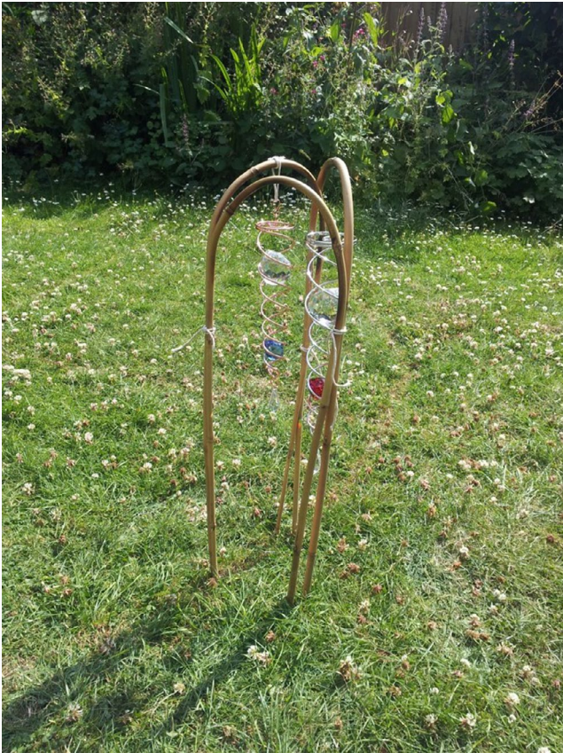
FIGURE 5 The object used for the neophobia test. The hanging ornaments spun in the wind and reflected light. DVDs were attached to the bamboo frame to increase reflectivity. The numerous sources of nocturnal light pollution (street lights, house lights, security lights, car lights, etc.) ensured that the neophobia stimulus was constantly changing day and night
