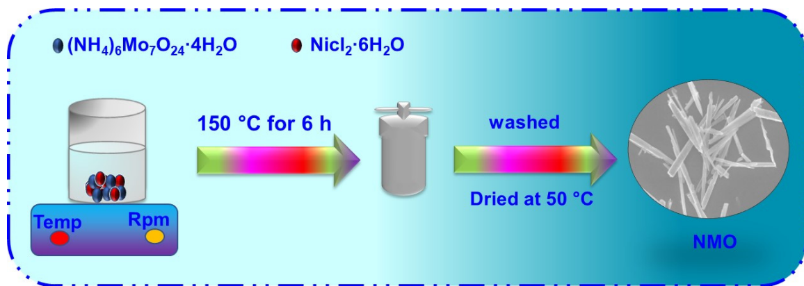
Scheme 1. Schematic Illustration of hydrothermal synthesis of NMO rods.
