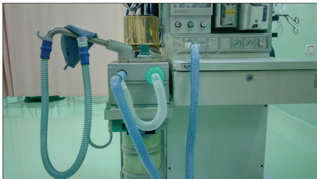
Figure 1: The Limb-O breathing circuit connected to the anaesthesia workstation
