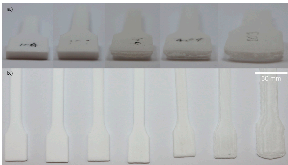
Figure 4. Optical micrographs of tensile test specimen. (a) Front perspective, from left to right with 5, 20, 25, 30, and 45% BL; (b) top perspective, from left to right with 5, 10, 15, 20, 25, 30, and 45% BL.
