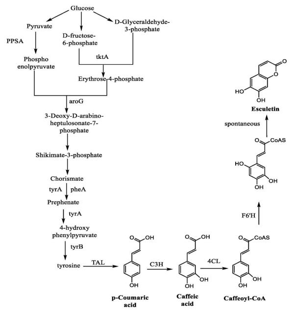
**Figure 11.** Synthesis of esculetin from glucose.
